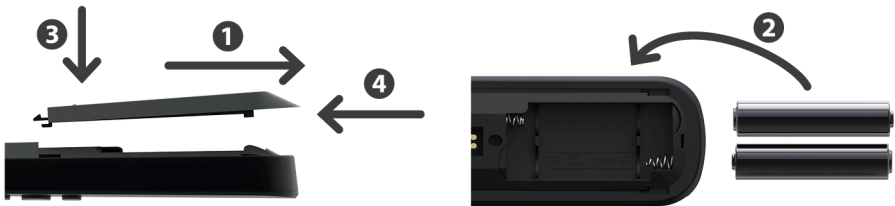
Figure 2: Inserting the batteries
